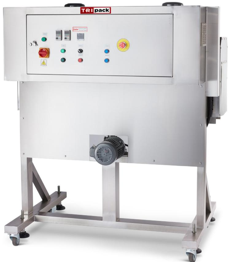
Tripack heat tunnels have adjustable baffles with digital temperature and variable air velocity controls to meet demanding shrink applications. This total shrink control gives you the ability to successfully shrink any sleeve application: tamper evident neck bands to full-body, high-shrink labels.
